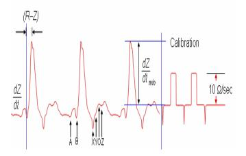
Table Timing of various notches in the first derivative impedance signal in impedance cardiography.
