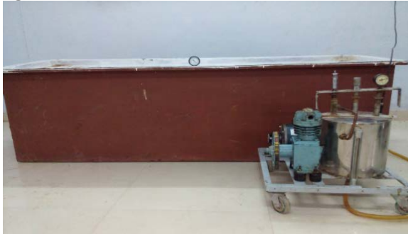
Figure-2: Steel vacuum chamber
